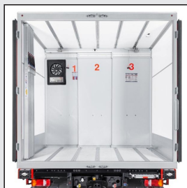
Cool Slide® as cold restraint system or dividing wall for multi-temp-transportation.
