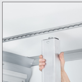
Load securing: Sturdy locking bars (up to 1000 daN)
