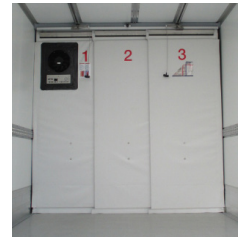
Cool Slide® - partition wall for transportation in several temperature zones
