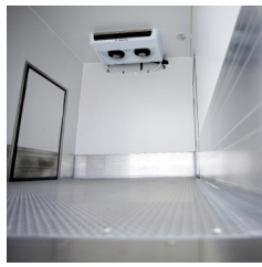
Liquid-tight floor tray made of aluminium barley grain
