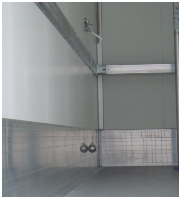
Picture 6: Measurement setup with 1 kg steel ball
