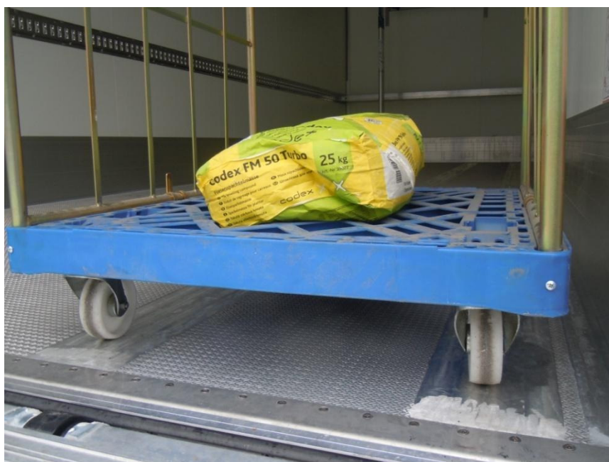
Picture 4: Quiet goods cart with 25 kg load on Kiesling low noise floor
